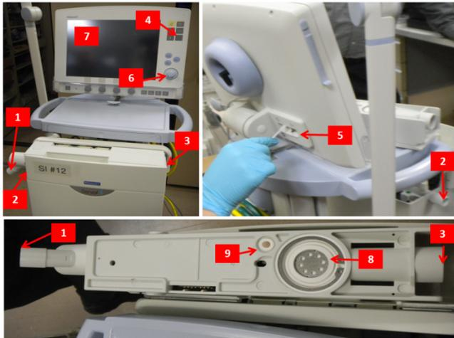
**Figure 1:** Nine reusable areas of the Maquet Servo Ventilator were swabbed to recover aerobic bacteria. The areas swabbed were: 1. Expiratory inlet, 2. Inspiratory outlet, 3. Exhaust port, 4. Interface buttons, 5. Power button, 6. Knob, 7. Screen, 8. Diaphragm, 9. Exhalation pressure port.
