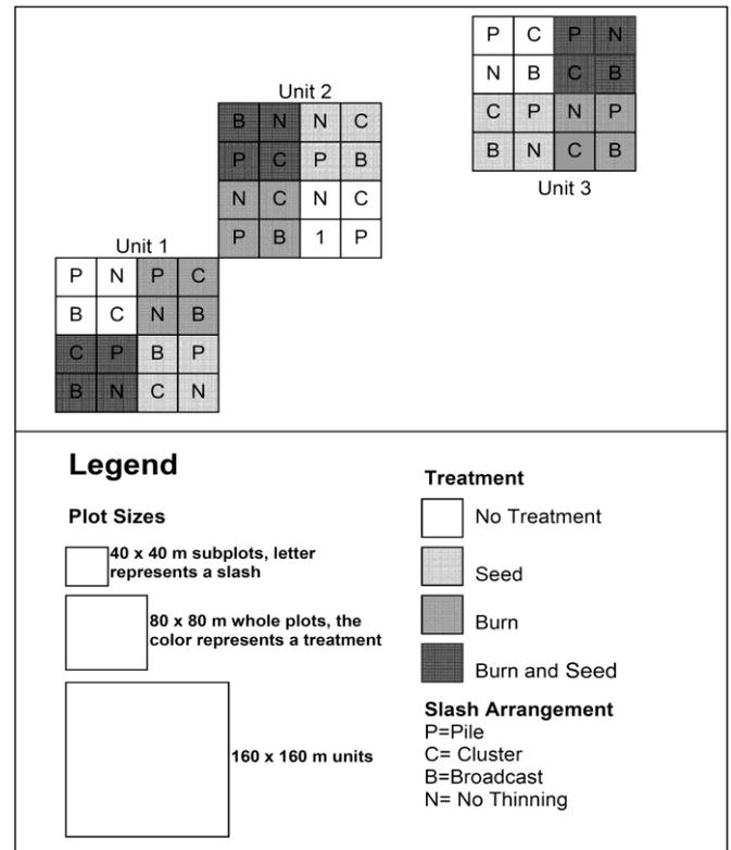
**Figure 1.** Split-plot experimental design replicated at each of the three sites.
