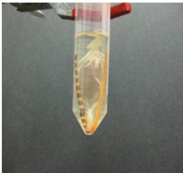
**Figure 1:** Picture of the test system: cells enclosed in dialysis tubing, placed in peanut oil with a device.
